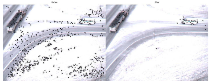
Fig. 7. Before image of all pixels and after image after ground plane pixels are segmented out
