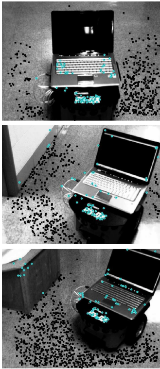
Fig. 6. Sample images from test sequences. Black squares are pixels classified as ground. Blue circles are pixels classified as non-ground.
