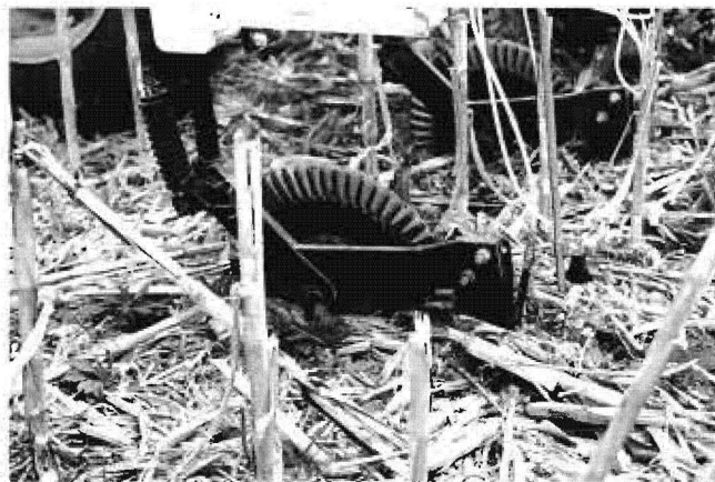
Figure 2. Knife injection of anhydrous ammonia or UAN solution is a best management practice for no-till nitrogen application.
