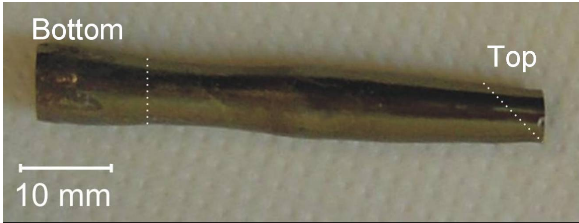
Fig. S1: Photograph of the single crystal as used in the initial HB3 experiment. For the initial HB3 experiment, the bottom part below the dotted line was masked with Gd paint, for subsequent DCS and HB3 experiments, the crystal was cut along the dotted lines.
