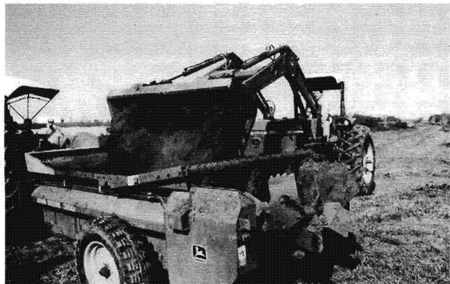
A front-end loader and beater-type spreader work well for loading and field-spreading compost.
