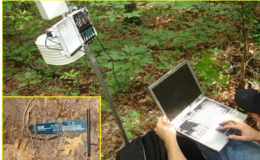
Figure 3.7- ECH 2 O® weather station located one each in both Angeline and Current River CA
