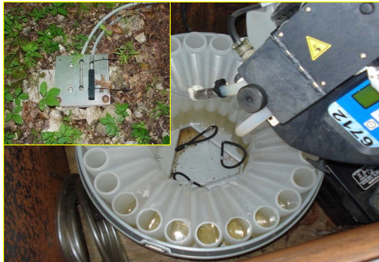
Figure 3.6- ISCO ® automated water sampler installed in A34-1 at the Angeline Conservation Area
