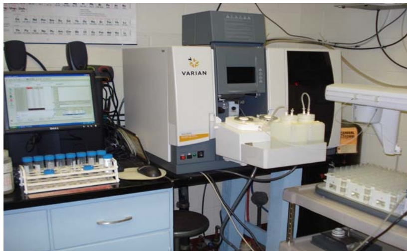
Figure 3.13- Varian 240FF Fast Sequential Atomic Absorption Spectrometer used to analyze Ca, Mg, K in the Soil Characterization Laboratory
