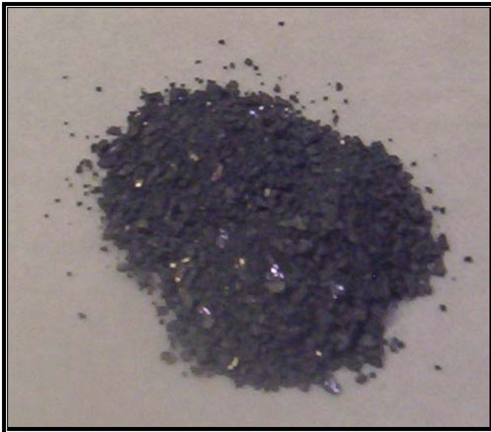
Figure.3.2: Al-nanoparticles coated with CTBN
