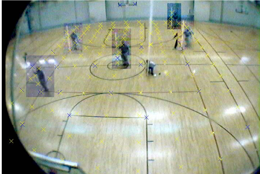
Figure 6.16 Marking Points by Nonlinear Model based on 22 Reference Points
