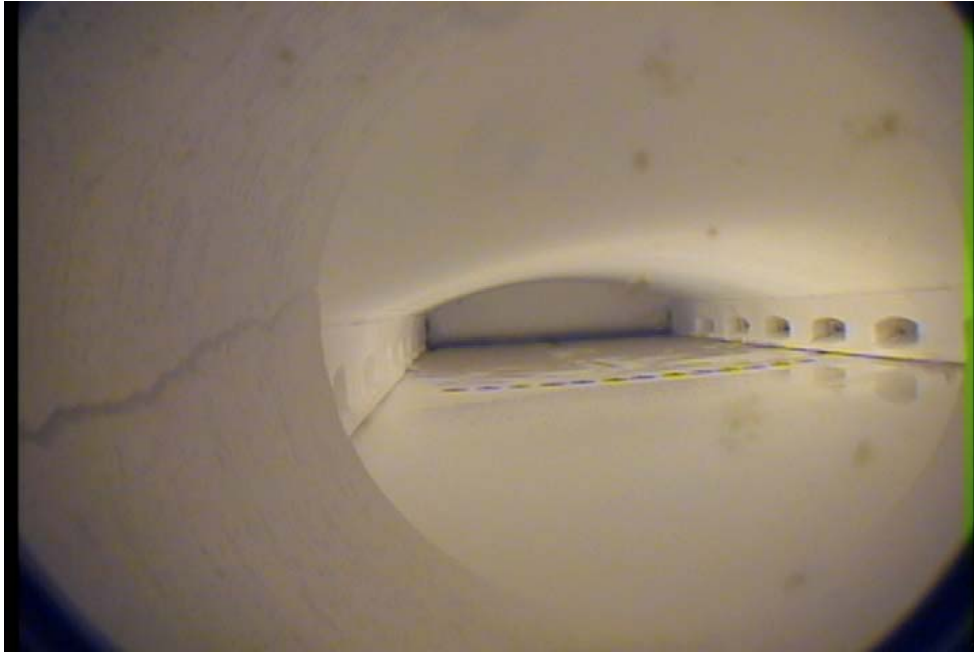
Figure 5.5 Furnace Image Captured by CCD Adjusted with the Wide Iris Position
