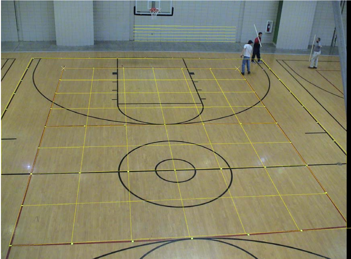
Figure 6.6 Redrawing Basketball Court by Linear Calibration Model
