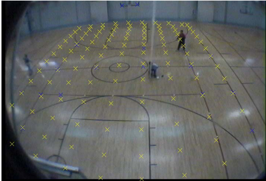
Figure 6.14 Marking Points by Nonlinear Model Based on 17 Reference Points
