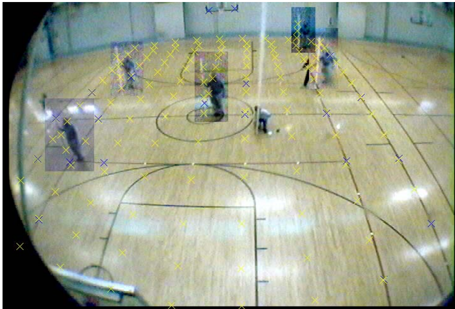
Figure 6.15 Marking Points by Nonlinear Model Based on 19 Reference Points
