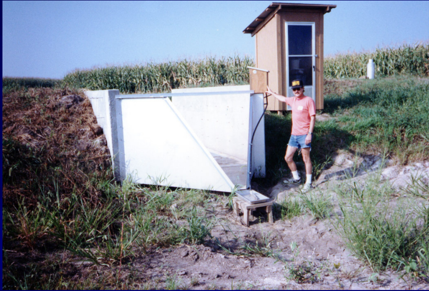
Sampler housing, concrete approach section, H-flume, and sample collection assembly
