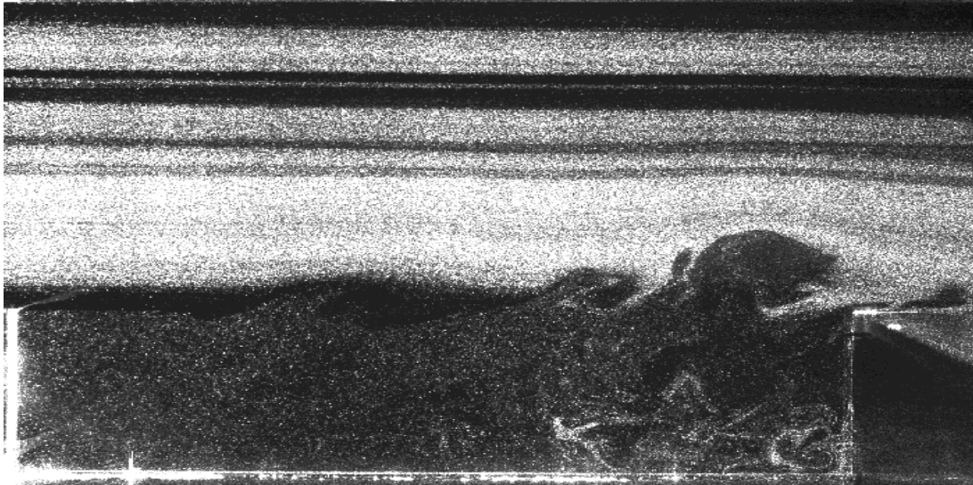
Figure 2.3: Flow visualization for a free stream velocity of 3 m/s ( Re_h=4000 )
