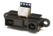
Figure 2.7: The Sharp GP2D12 infrared range finder
