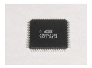
Figure 2.18: ATMEL ATmega128
