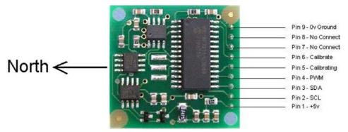
**Figure 2.13:** The Devantech CMPS03 compass module
