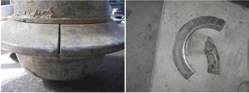
Figure 7.2.1: Laser cracks on disc cutters
