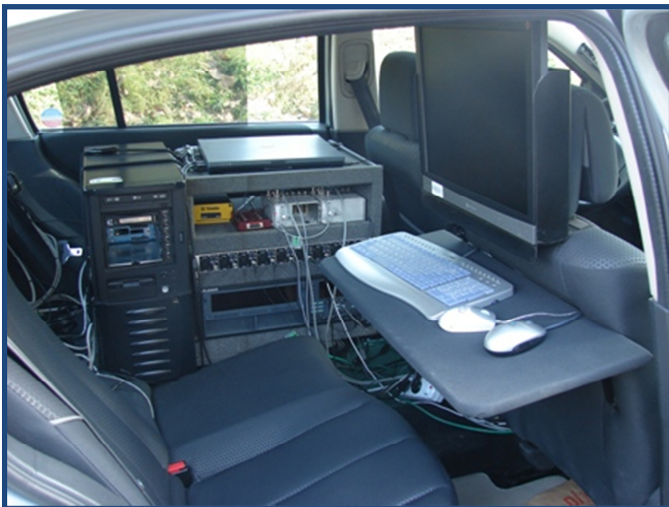
Figure 3.3 : A photo from the interior of data acquisition car.
