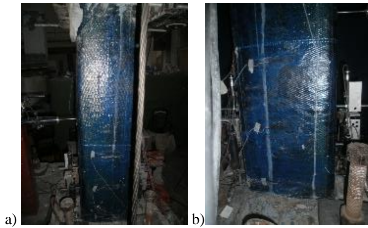
Figure B.50 : a) North, and b) South view of X26-M-CFRP1 after -6.00% mm drift ratio.
