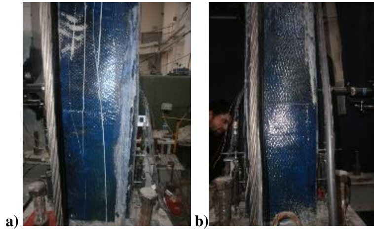
Figure B.55 : a) North, and b) South view of X43-M-CFRP2 after -0.5% mm drift ratio.
