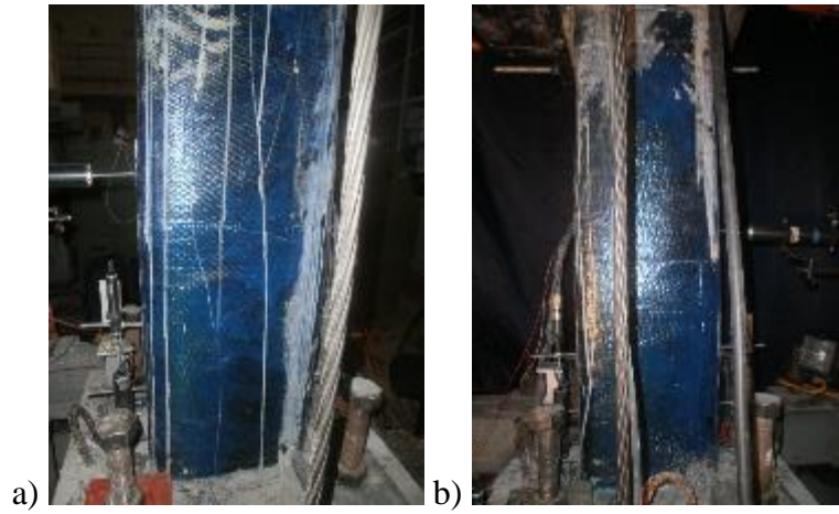
Figure B.61 : a) North, and b) South view of X43-M-CFRP2 after -3.00% mm drift ratio.
