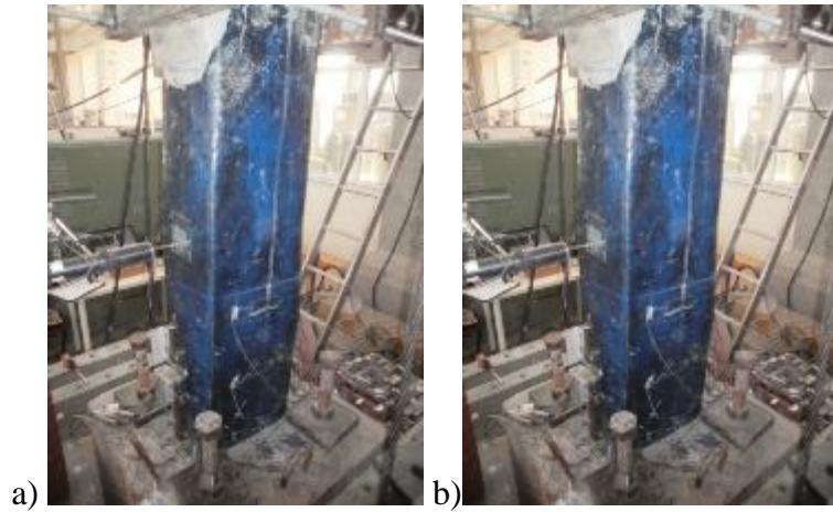
Figure B.43 : a) North, and b) South view of X26-M-CFRP1 after -2.00% mm drift ratio.
