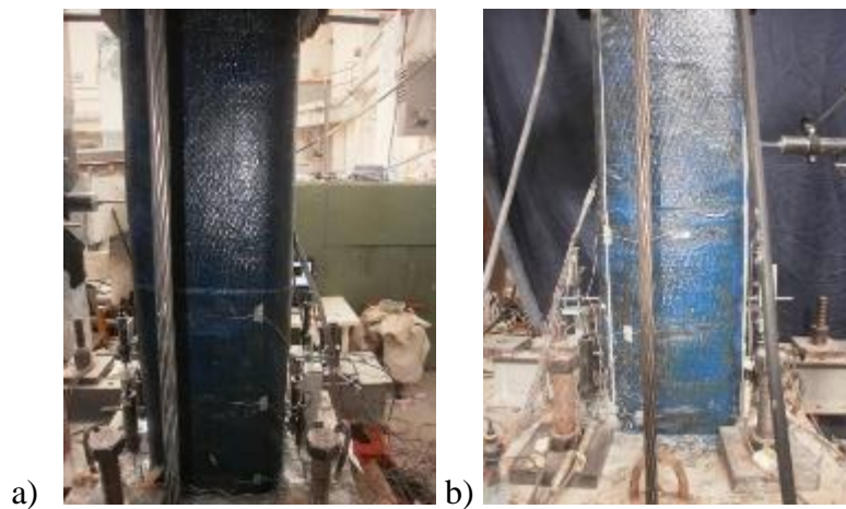
Figure B.72 : a) North, and b) South view of X44-M-CFRP3 after -2.00% mm drift ratio.
