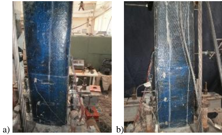
Figure B.40 : a) North, and b) South view of X26-M-CFRP1 after -0.75% mm drift ratio.
