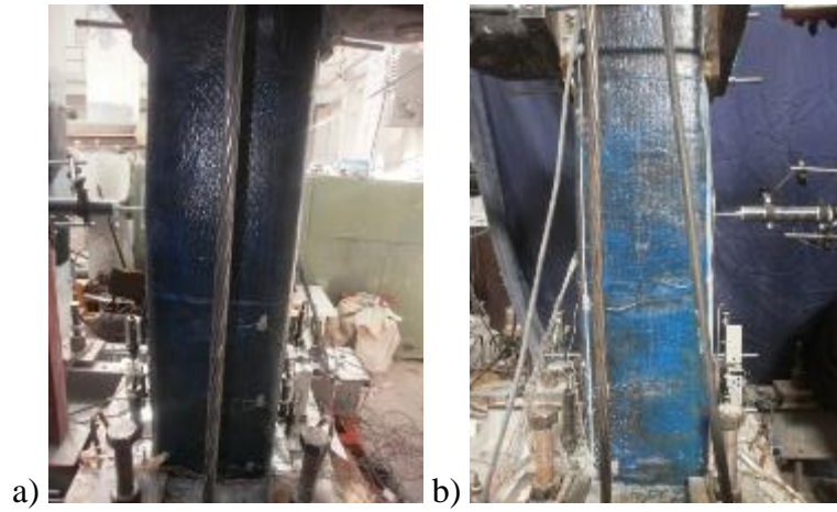
Figure B.67 : a) North, and b) South view of X44-M-CFRP3 after -0.25% mm drift ratio.
