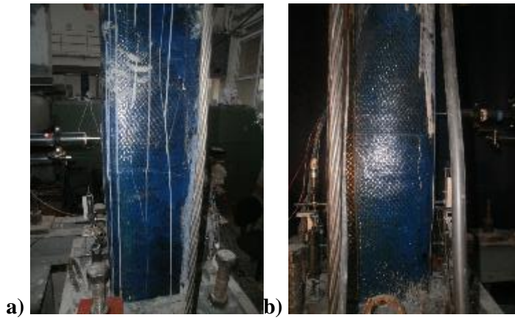
Figure B.58 : a) North, and b) South view of X43-M-CFRP2 after -1.50% mm drift ratio.
