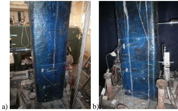
Figure B.46 : a) North, and b) South view of X26-M-CFRP1 after -3.50% mm drift ratio.
