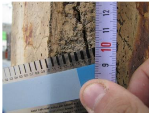
Figure 5.1 : Crack measuring of the specimen.
