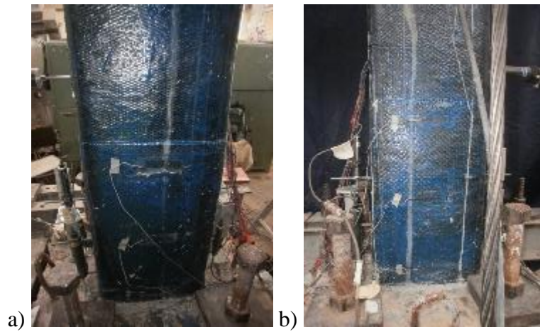
Figure B.38 : a) North, and b) South view of X26-M-CFRP1 after -0.25% mm drift ratio.
