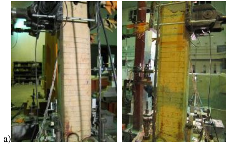
Figure B.16 : a) North, and b) South view of X26-REF2 after -1.50 % mm drift ratio.
