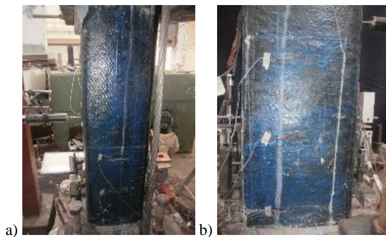
Figure B.39 : a) North, and b) South view of X26-M-CFRP1 after -0.5% mm drift ratio.
