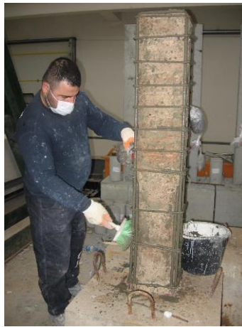
Figure 5.4 : Specimens were covered with a corrosion inhibitor material.
