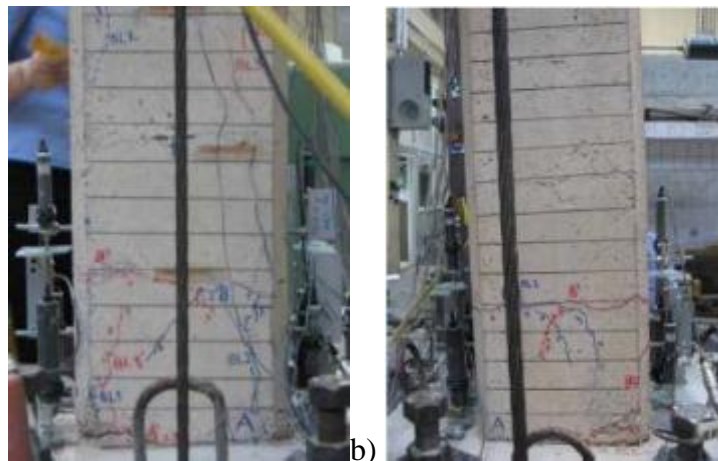
Figure 7.3 : a) North, and b) South view of the LS-C0 specimen after -3.50% drift ratio (Goksu, 2012).
