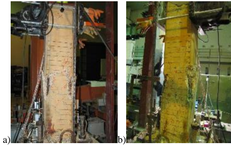
Figure B.19 : a) North, and b) South view of X26-REF2 after -3.00 % mm drift ratio.
