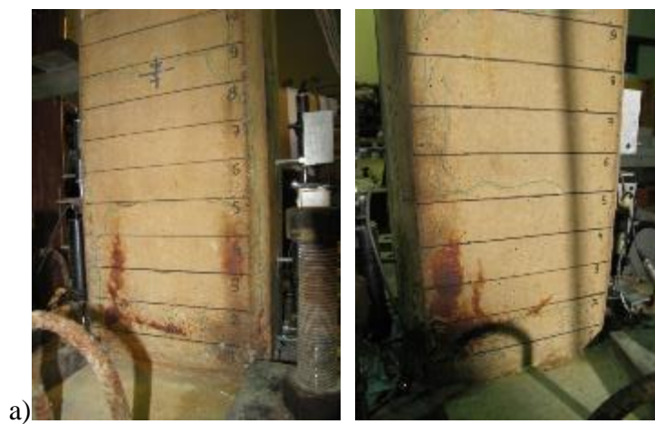
Figure B.12 : a) North, and b) South view of X26-REF2 after -0.25% mm drift ratio.
