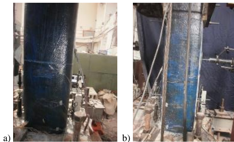
Figure B.69 : a) North, and b) South view of X44-M-CFRP3 after -0.75% mm drift ratio.
