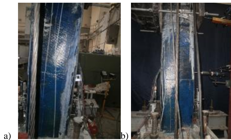
Figure B.63 : a) North, and b) South view of X43-M-CFRP2 after -4.00% mm drift ratio.
