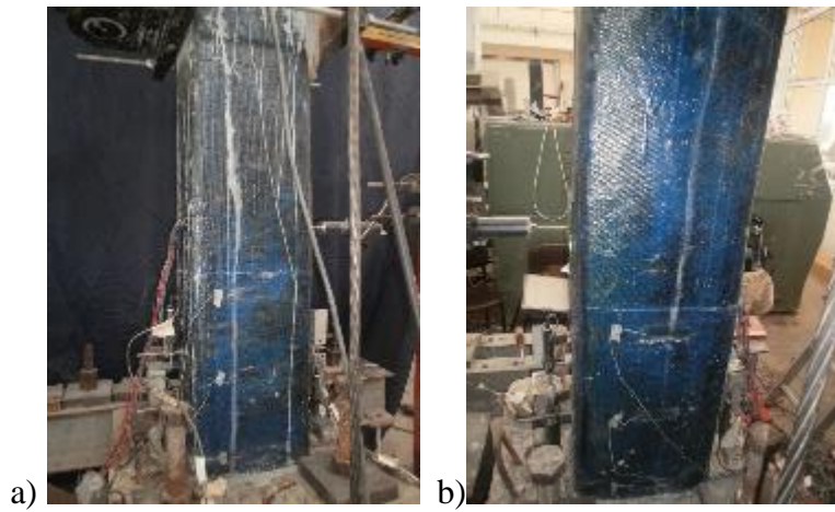
Figure B.41 : a) North, and b) South view of X26-M-CFRP1 after -1.00% mm drift ratio.
