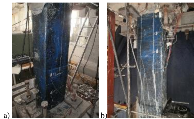
Figure B.42 : a) North, and b) South view of X26-M-CFRP1 after -1.50% mm drift ratio.
