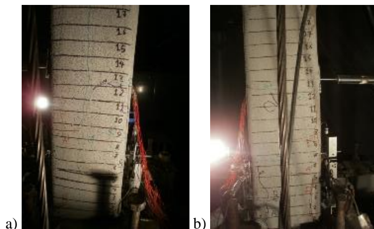
Figure 7.26 : a) North, and b) South view of X26-M after -4.00 % mm drift ratio.
