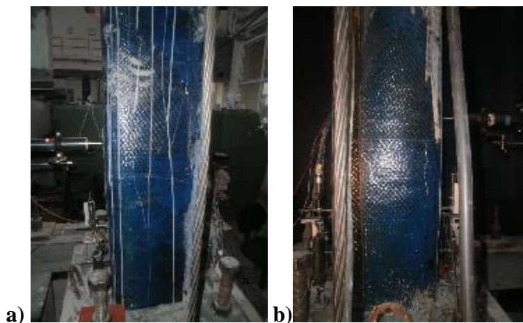
Figure B.60 : a) North, and b) South view of X43-M-CFRP2 after -2.50% mm drift ratio.
