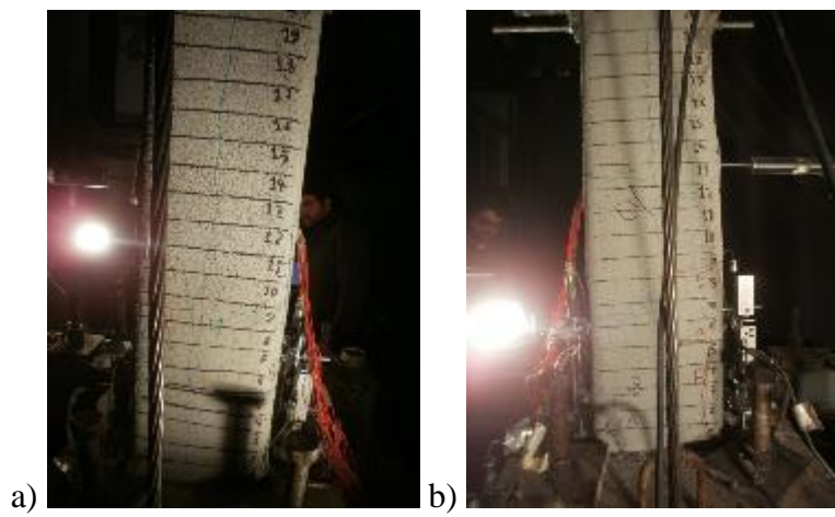
Figure B.30 : a) North, and b) South view of X26-M after -3.50 % mm drift ratio.
