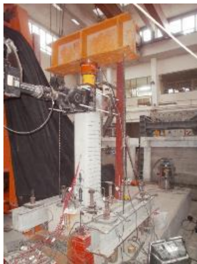
Figure 7.21 : The view of the specimen X26-M before the starting of test
