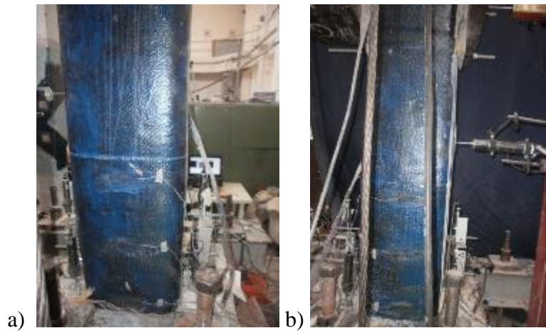
Figure B.68 : a) North, and b) South view of X44-M-CFRP3 after -0.5% mm drift ratio.
