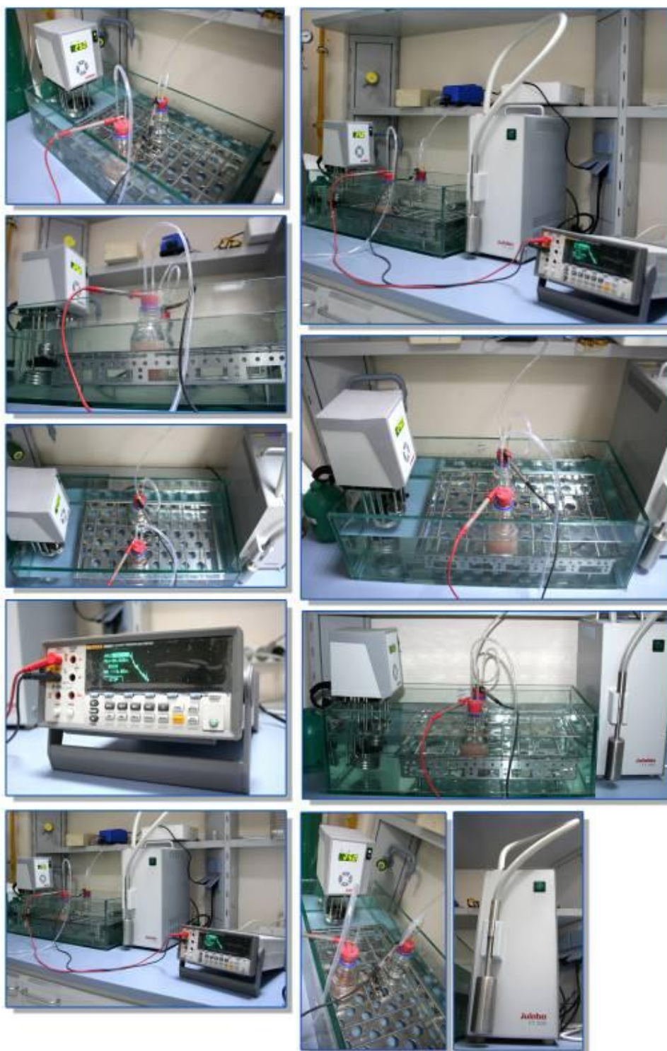
Figure 3.5: Two chambered MFC used.
