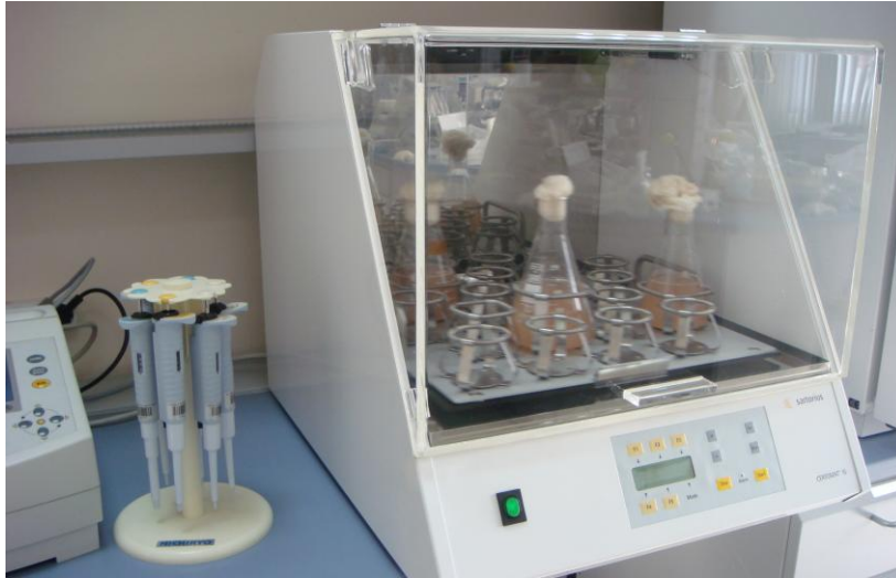
Figure 3.1: Sartorius Certomat IS cooling rotary shaker.
