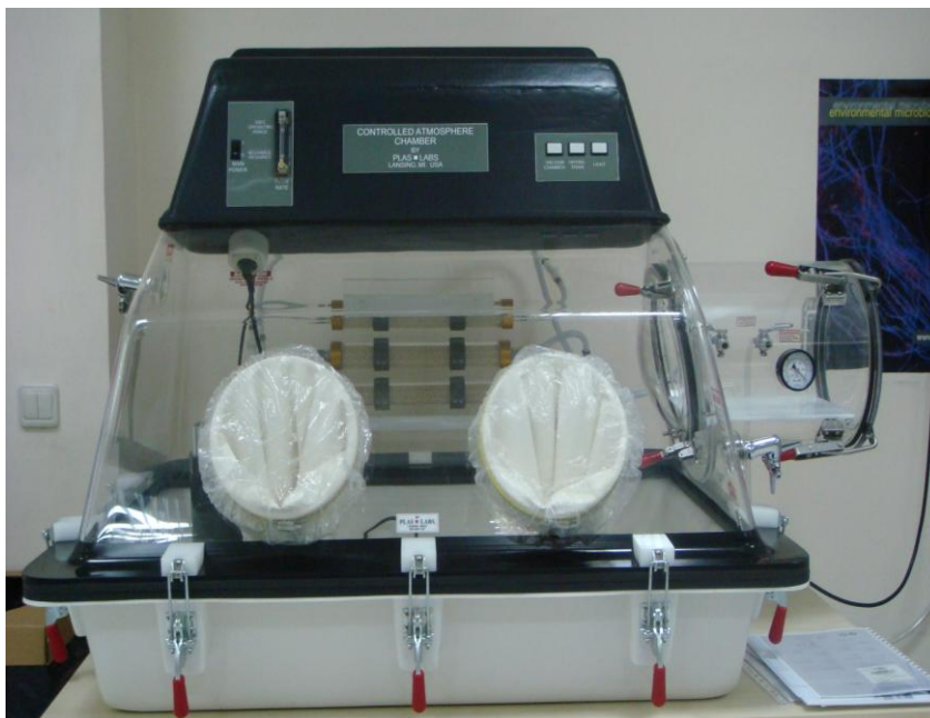
Figure 3.2: Controlled Atmosphere Chamber(PLAS LABS USA).
