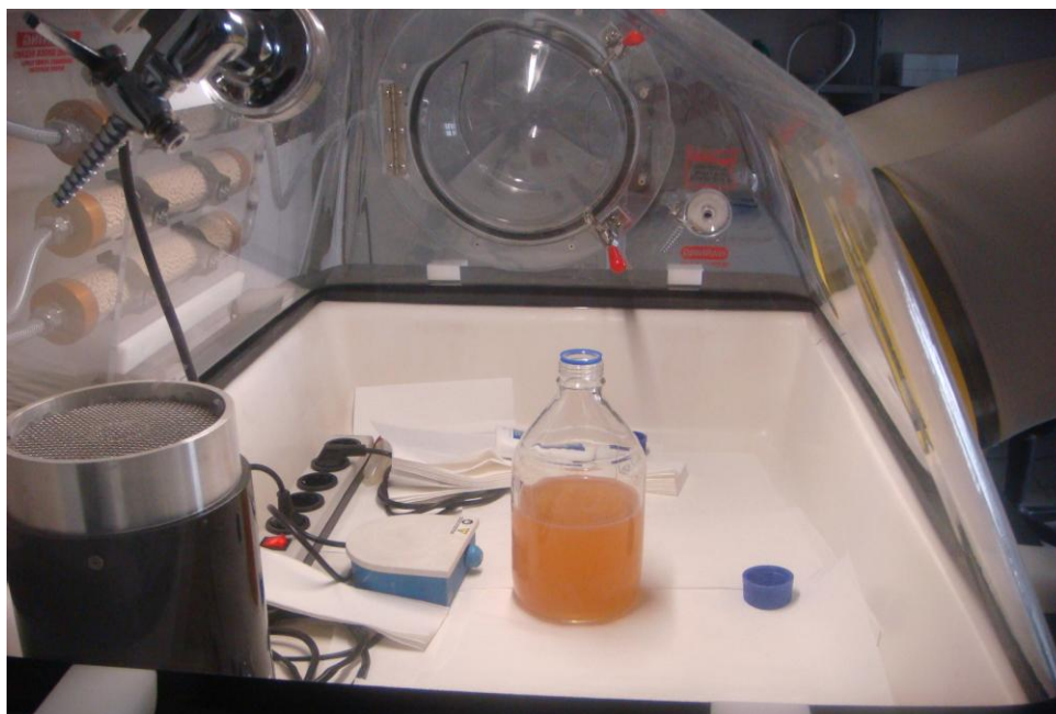
Figure 3.3: Anoxic growth of S.putrefaciens in Atmosphere Controlled Chamber. LB (MILLER) broth in glass bottle was inoculated with 12.5 ml of an aerobically grown overnight culture and incubated without agitation. After 96 hrs of growth, the cells were harvested under anoxically conditions by a continuous centrifugation system (Hettich Rotina 420 R Centrifuge) at 4800 rpm at 4°C (Figure 3.4)
