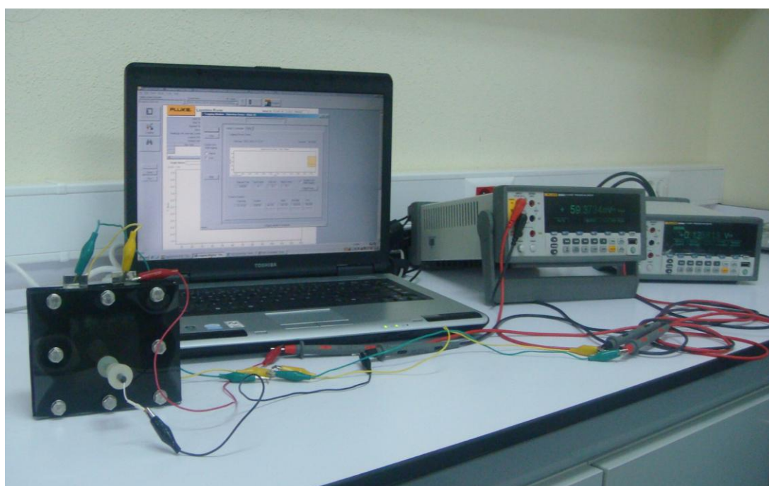
Figure 3.9: Photograph of SCF-2-MFC connecting multimeter system.
