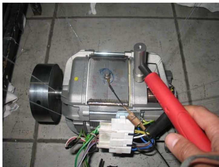
Figure 3. 12 : Locations of impact force and acceleration response of hanged motor.
