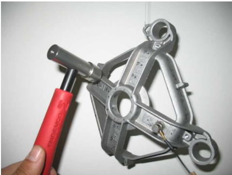
Figure 3. 2 : Locations of impact force and acceleration response for the front cover.
