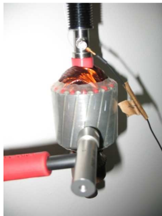
Figure 3. 8 : Locations of impact force and acceleration response of rotor.
