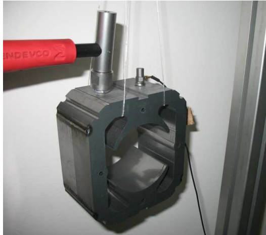
Figure 3. 6 : Locations of impact force and acceleration response of stator.
