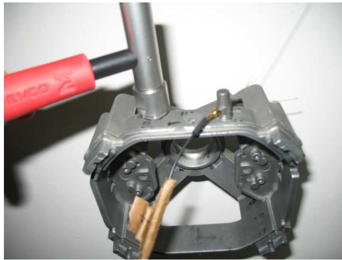
Figure 3. 4 : Locations of impact force and acceleration response of rear cover.
