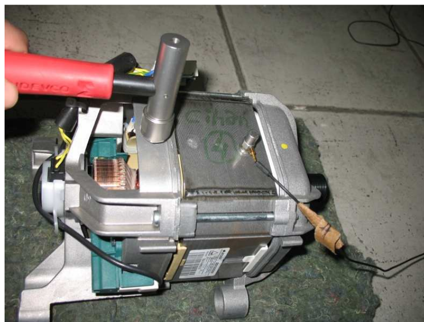
Figure 3. 10 : Locations of impact force and acceleration response of motor.
