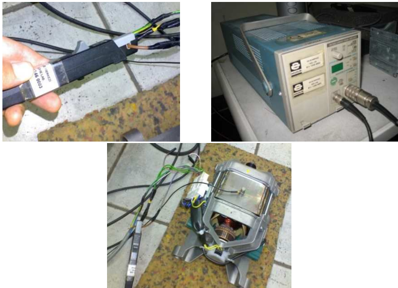
Figure 3.17 : Current measurement set-up.
