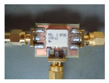
Figure 3.21 : SYM-11 double-balanced frequency mixer.
