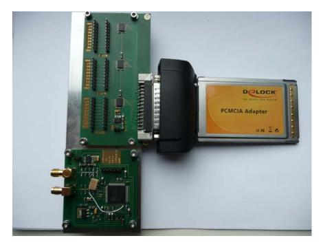
Figure 3.5 : AD9910 application board.
