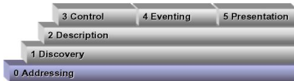
Figure 3.10: UPnP Networking Procedure
