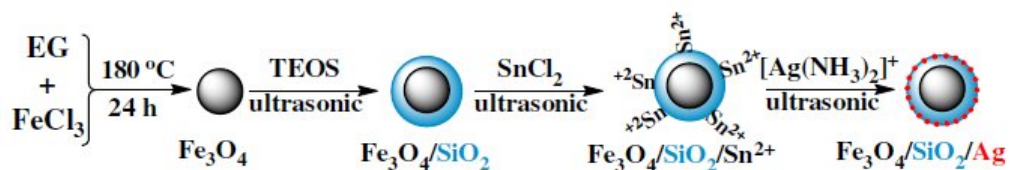
Figure 1.6 : Purposed diagram for the synthesis of magnetite multifunctional NPs (Lv et al, 2010).
