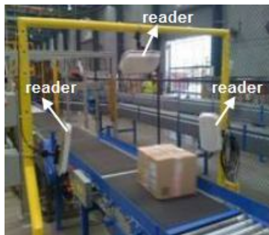
Figure 3.18 : RFID tagged packages of mobile phones moving on RFID-enabled packaging line (Friedlos, 2009).
