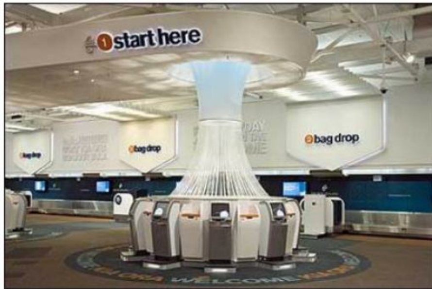
Figure 3.12 : Air New Zealand's RFID-enabled kiosks where passengers use their ePass to check in themselves (Friedlos, 2008b).
