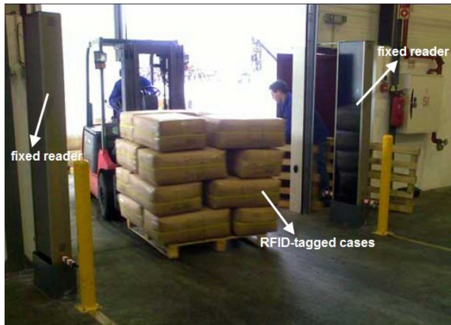
Figure 3.19 : RFID-tagged cases of material is being brought through a portal reader at Marigold Industrial Plant (O'Connor, 2009).
