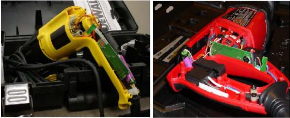
Figure 3.5 : Tools that are installed with active RFID tags (Goodrum et al., 2006).
