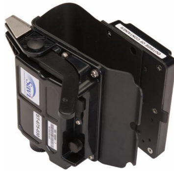
Figure 3.14 : Sensor integrated active RFID tags used at container doors for intrusion detection (Url-28).
