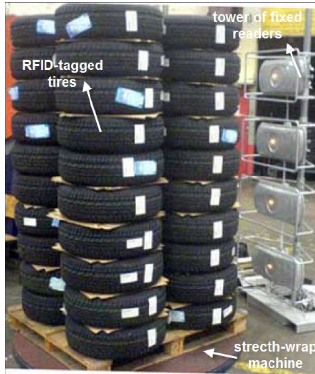
Figure 3.17 : RFID-tagged tire stacks on a stretch-wrap machine prepared for a customer order (Wessel, 2009c).
