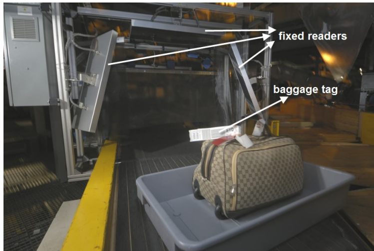
Figure 3.8 : RFID-enabled baggage handling system at the HKIA (Url-9).
