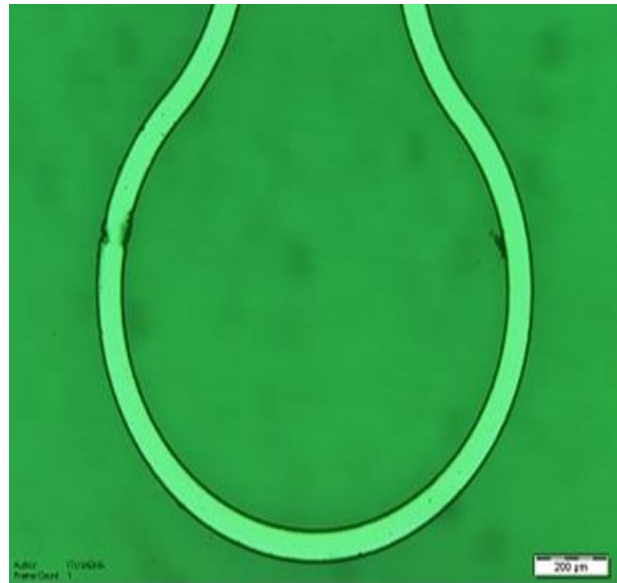
Figure 3.5 : Optical microscope image of a defected channel.
