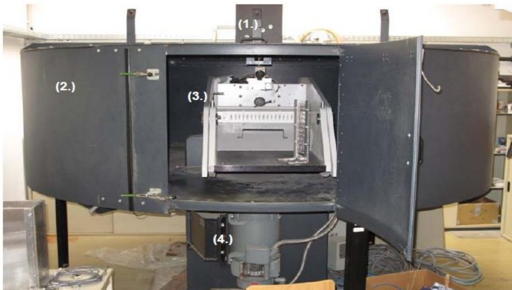
Figure 4.3 : IGT beam centrifuge: (1.) slip ring tower, (2.) high strength steel enclosure, (3.) rotating arm, (4.) DC motor (Idinger,2010)
