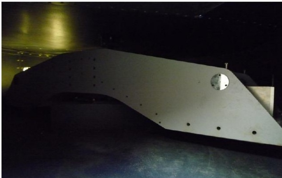
Figure 4.4 : Rotating beam - model at the back and box with counterweights at front (Idinger,2010)
