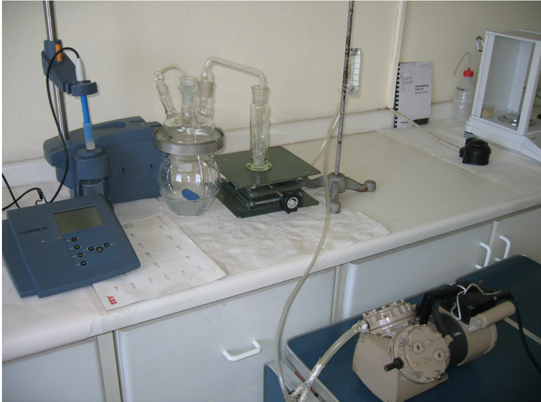
Figure 4.4: Picture of stripping/absorption unit.
