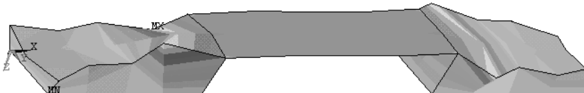
Figure A.2 : Mode shapes of the bridge (10-17).
