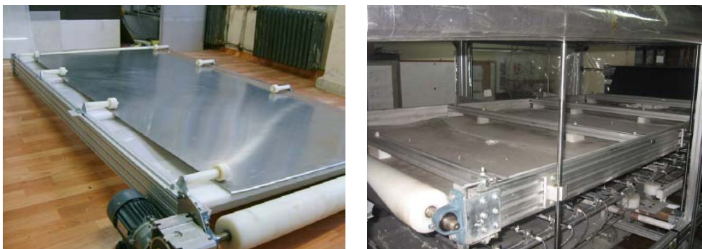
Figure 5.19 : Conveyor system as collector.
