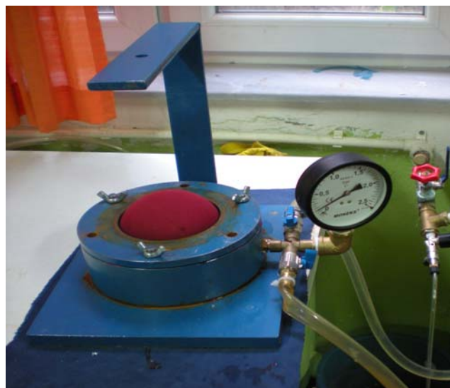
Figure 3.9 : Test apparatus for resistance to water penetration.
