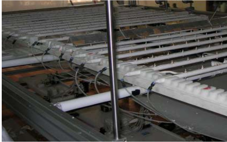
Figure 5.35 : PTFE pipe-needle block in pilot unit.
