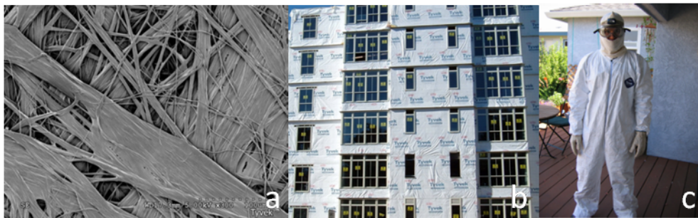
Figure 3.3 : Tyvek ® water resistant breathable fabric a) SEM photograph of Tyvek ® b)Tyvek ® weather barrier c) Tyvek ® protective apparel [83-85].
