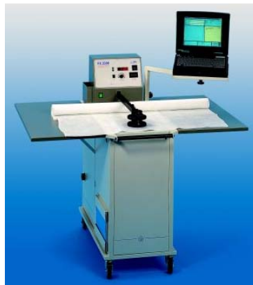
Figure 3.11 : Textest Fx 3300-III air permeability tester [97].
