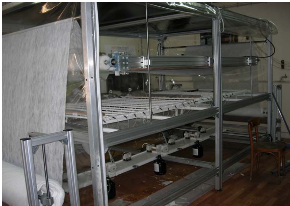
Figure 5.25 : Photograph of assembled pilot electrospinning unit.
