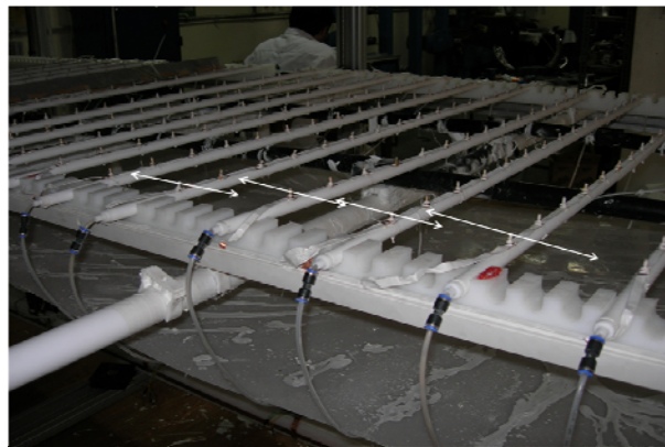
Figure 5.26 : Pipe-needle layout in electrospinning pilot unit.
