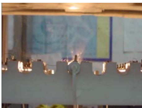
Figure 5.27 : Electrospinning jets during electrospinning.
