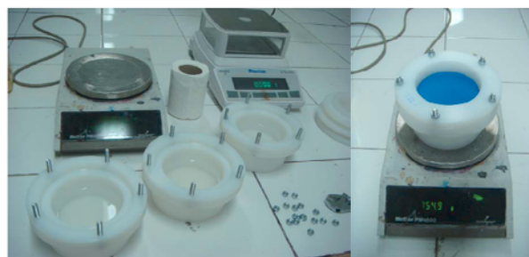
Figure 3.10 : Test dishes for water vapor transmission.
