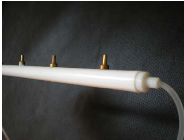
Figure 5.15 : PTFE pipe-needle solution transfer system.
