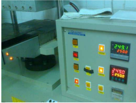
Figure 3.3: Temperature control panel and pressure gauge of hydraulic hot press instrument.
