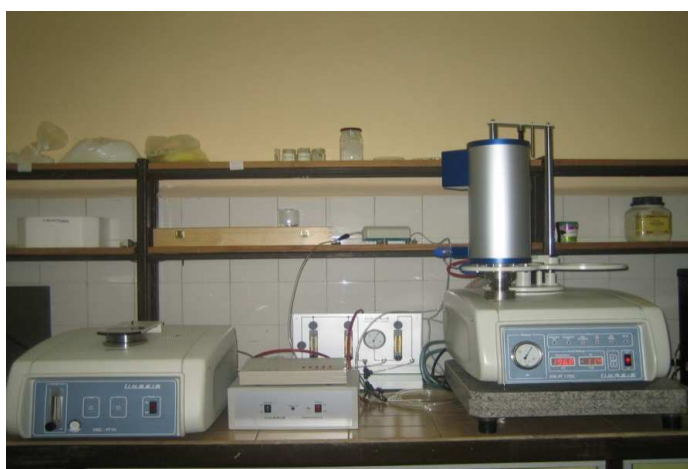
Figure 3.7 : Linseis STA PT 1750 model TGA/DTA combined instrument.
