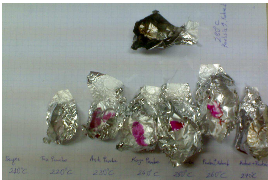
Figure 3.12 : Decomposition behaviour of 5-PT with increasing temperature.
