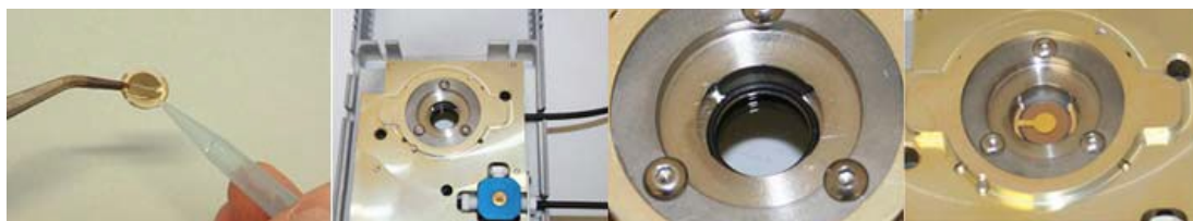
Figure 3.3: The insertion of o-ring and quartz crystals.
