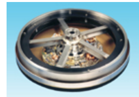
Momentum and Reaction Wheel RSI 68 14-68 Nms with integrated Wheel Drive Electronics
