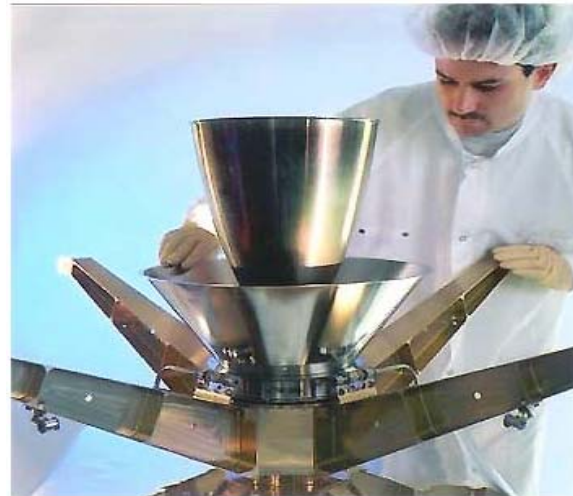
Integration of 400 N apogee engine and heat shield to thrust frame.
