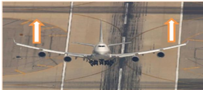
Figure 1.2 : Deformation of wing due to aerodynamic loads
