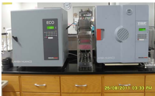
Figure 3.4: Ahiba Nuance machine used for scouring of the fabric samples.
