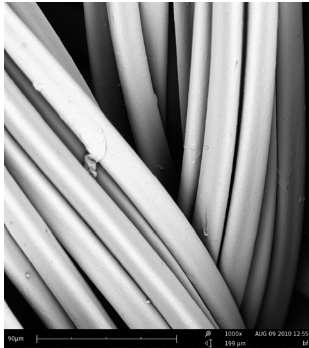
Figure 4.25: SEM images for treated flat warp knitted samples with silver nitrate antimicrobial agent; (Magnification X1000).
