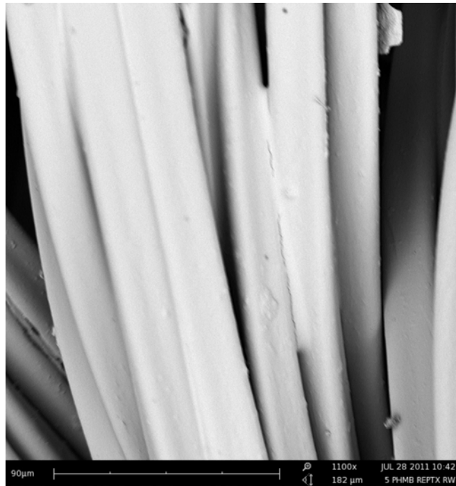
Figure 4.40: SEM images for treated flat warp knitted fabric samples with PHMB antimicrobial chemical agent; (Magnification X1100).
