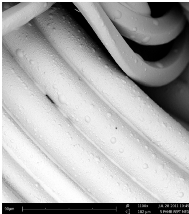
Figure 4.41: SEM images for treated weft knitted fabric samples with PHMB antimicrobial chemical agent; (Magnification X1100).
