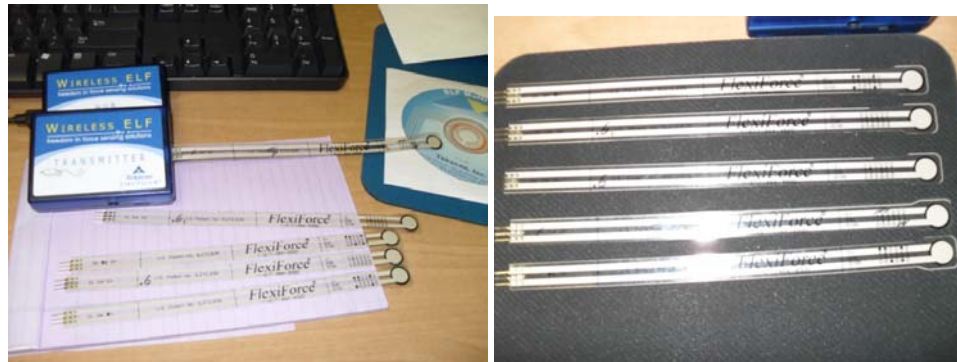
Figure 3.11: Wireless pressure sensors used for pressure measurements.
