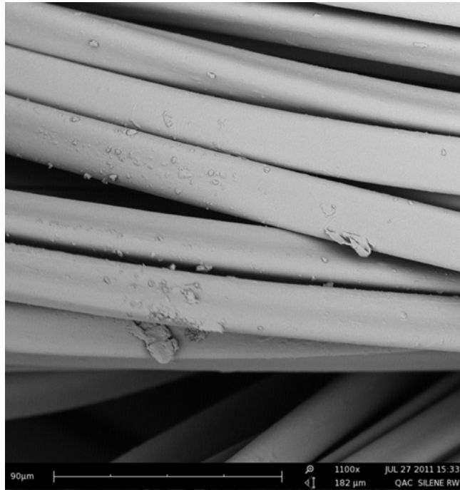
Figure 4.28: SEM images for treated flat warp knitted fabric samples with Quat Silane antimicrobial agent; (Magnification X1100).
