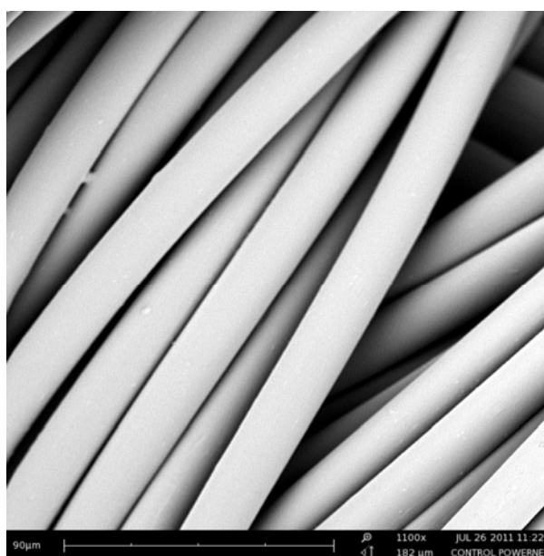
Figure 4.21: SEM Images for untreated powernet warp knitted fabric samples (Magnification X1100).
