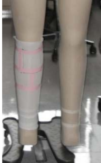
Figure 3.10: Static mannequin and pressure garments designed for leg (from ankle to knee).
