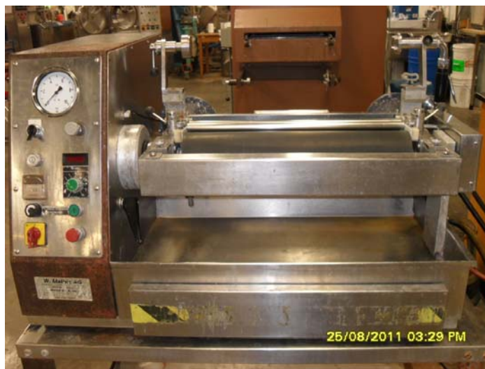
Figure 3.6: Mathis HVF padder used for the antimicrobial treatments.
