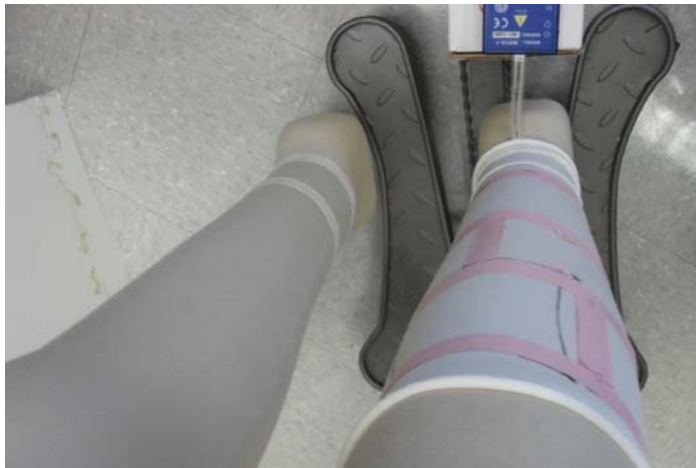
Figure 3.31: Taking pressures from ankle by wireless pressure sensors.
