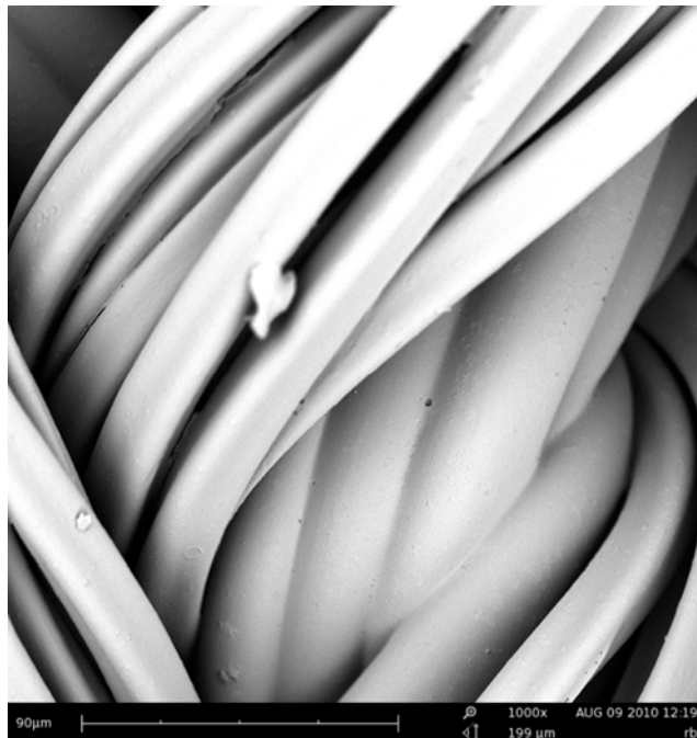
Figure 4.26: SEM images for treated weft knitted fabric samples with silver nitrate antimicrobial agent; (Magnification X1000).
