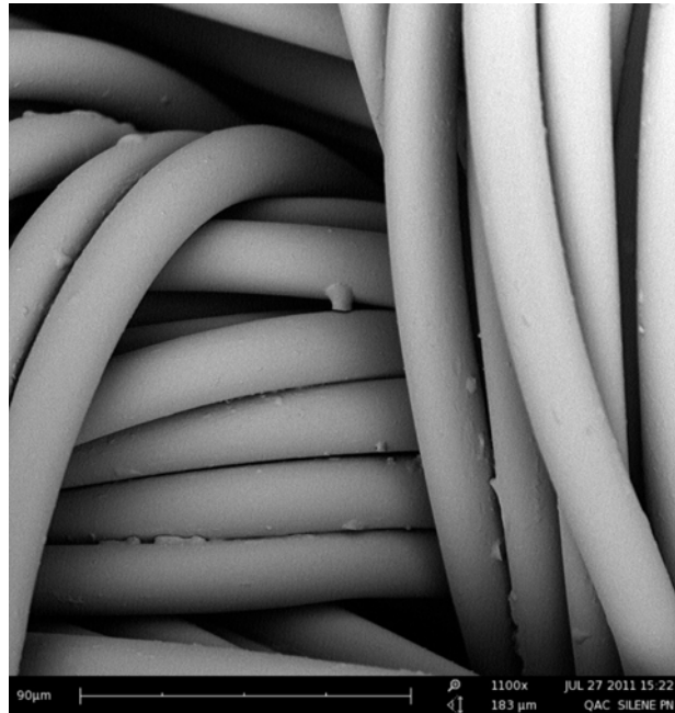
Figure 4.27: SEM images for treated powernet warp knitted fabric samples with Quat Silane antimicrobial agent; (Magnification X1100).
