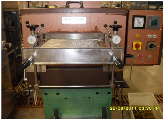
Figure 3.9: Mathis LTF stenter used for the curing of the samples.
