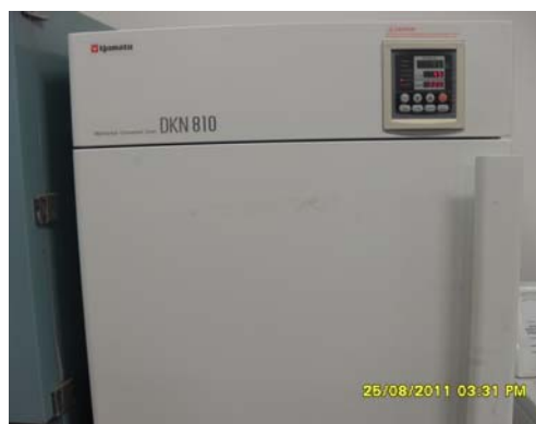
Figure 3.8: Yamato convection oven used for the drying of the fabric samples.
