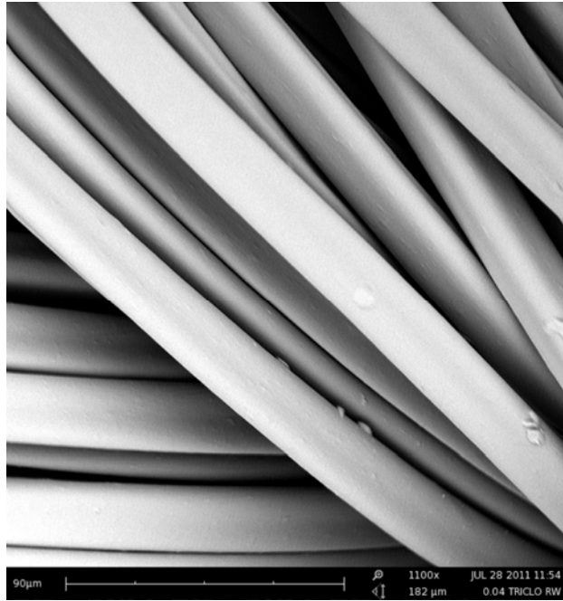
Figure 4.34: SEM images for treated flat warp knitted fabric samples with Triclosan antimicrobial agent; (Magnification X1100).
