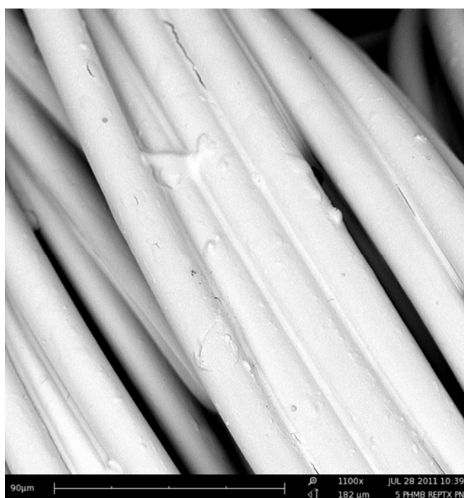
Figure 4.39: SEM images for treated powernet fabric samples with PHMB antimicrobial chemical agent; (Magnification X1100).
