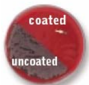
Figure 2.10: Microbial growth in uncoated sample and sample coated with PVA as a carrier (14 Days) [175].
