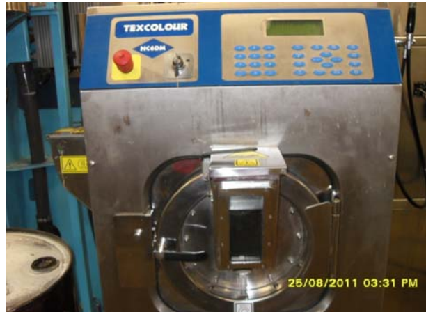
Figure 3.5: Texcolour machine used for scouring of the fabric samples.
