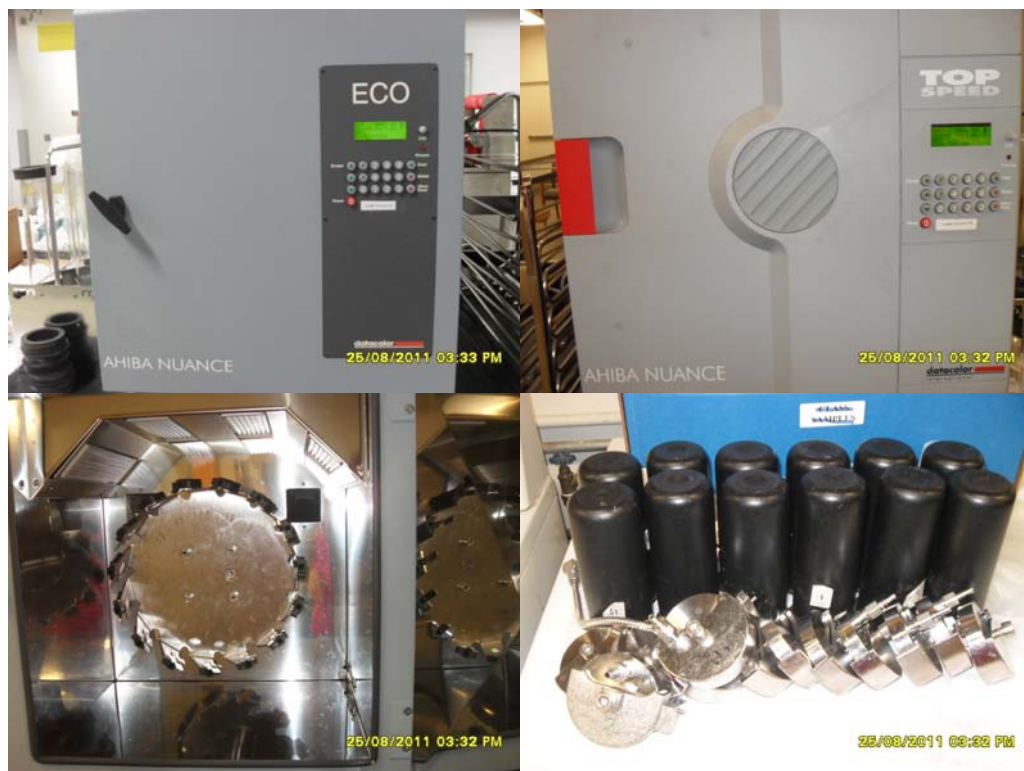
Figure 3.7: Ahiba Nuance machine used for antimicrobial treatment of the fabric samples.
