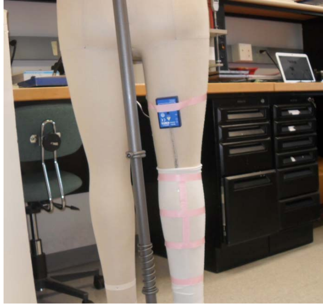
Figure 3.30: Taking pressures from calf by wireless pressure sensors.
