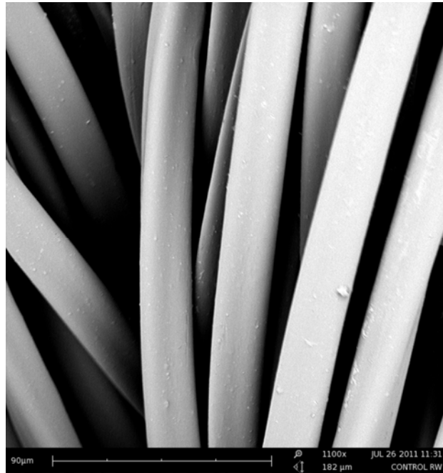
Figure 4.22: SEM images for untreated flat warp knitted fabric samples; (Magnification X1100).
