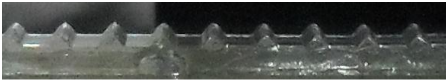
Figure 4.9 : Front-view of the artificial skin made of PDMS which is the positive of the mold.
