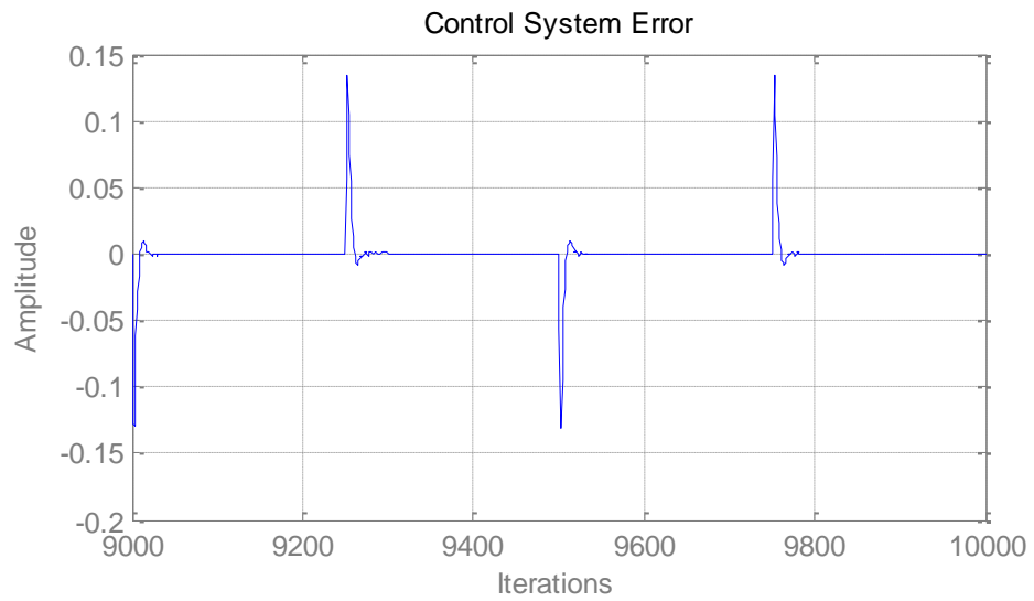
Figure 7.5 Overall control system error of time-invariant plant
