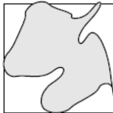
Figure 2.11: Axis Aligned Bounding Box
