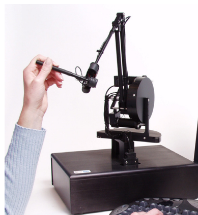
Figure 4.6: Phantom Premium Desktop Device
