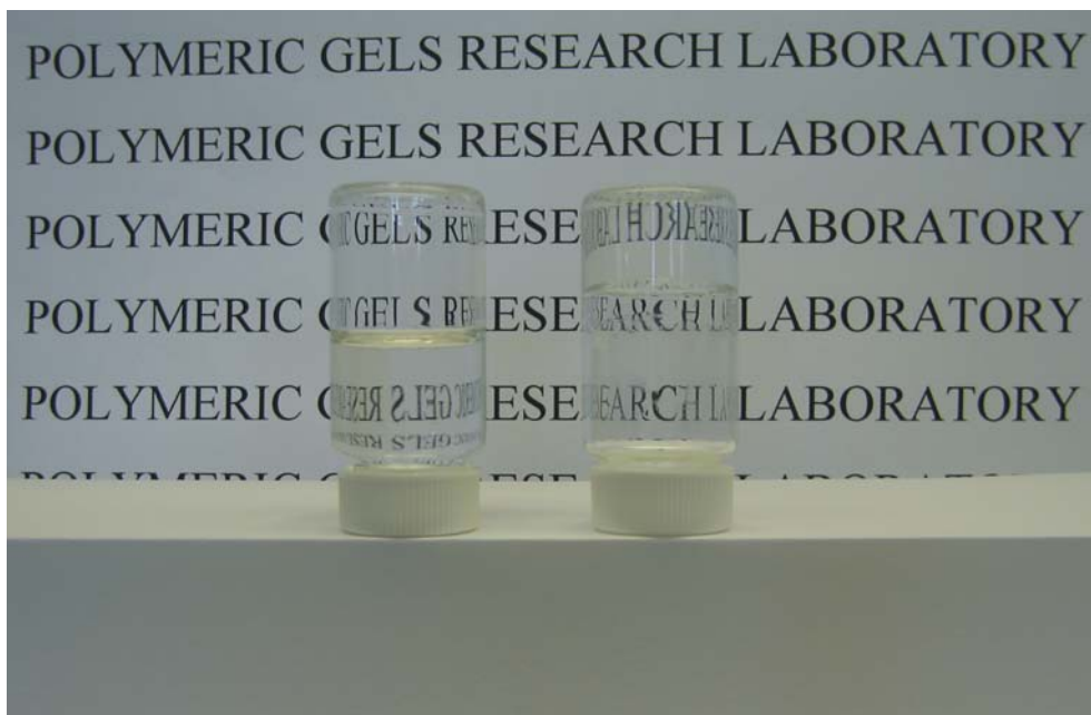
Figure 1.2: Photographs of the polymer solution (left) and the gel sample (right).
