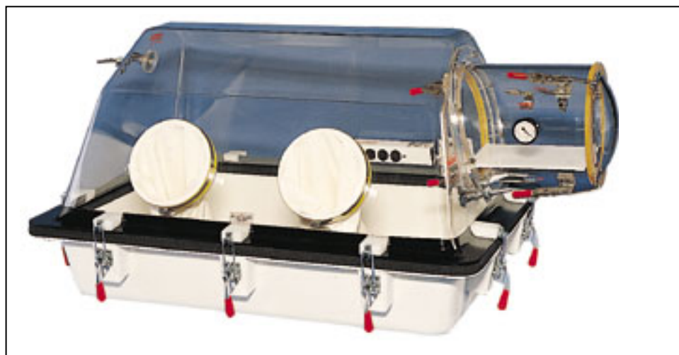
Figure 5.2: Dust-free glovebox used in the experiments.
