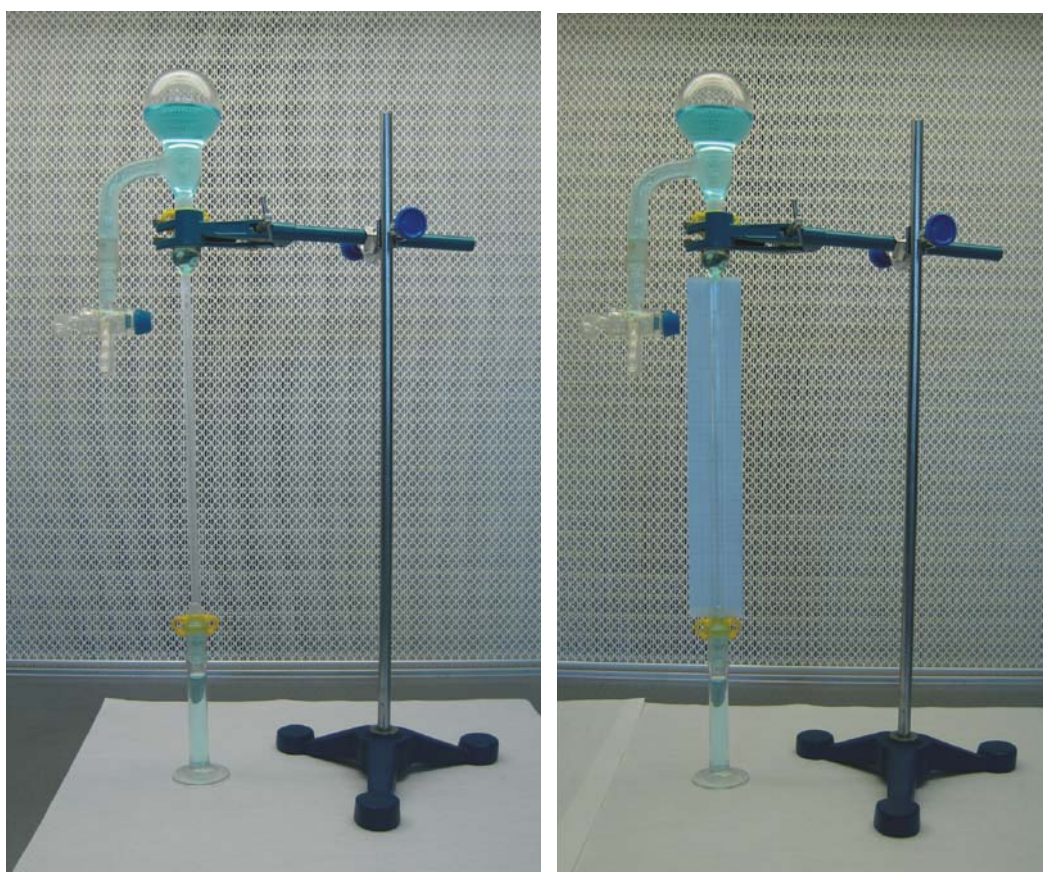
Figure 5.11: The dilatometer consisting of a blown glass bulb connected to a 30 cm length of 1.5 mm precision-bore capillary tubing (left). A millimetric paper was connected to capillary tubing (right).
