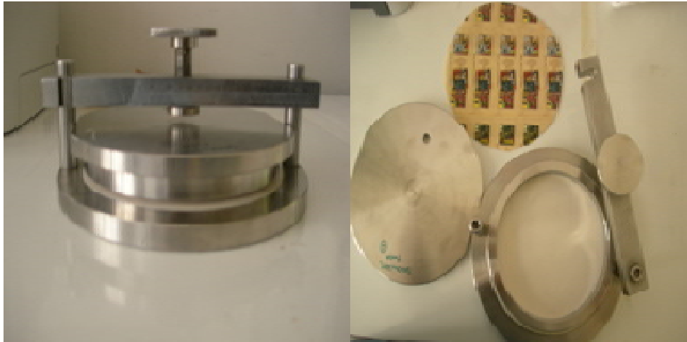
Figure 3.2 : Commercial migration cell used in the test.
