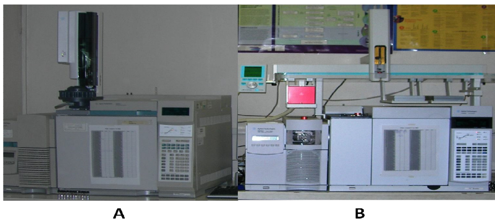
Figure 3.1 : A) GC system equipped with an auto-injector and HP 5973 mass-selective detector (Agilent Technologies, Palo Alto, USA), B) Solid phase microextraction (SPME) adopted with GC/MS(Agilent Technologies, Palo Alto, USA)
