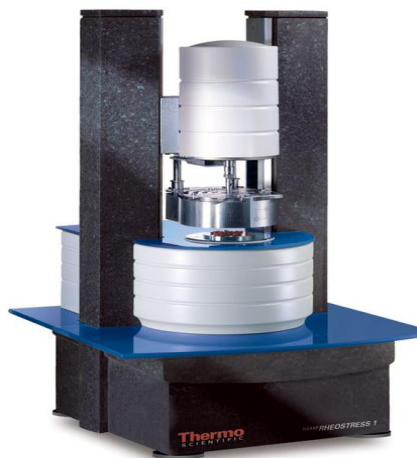
Figure 6.2: Rheometer setup (HAAKE Rheostress 1, Germany).
