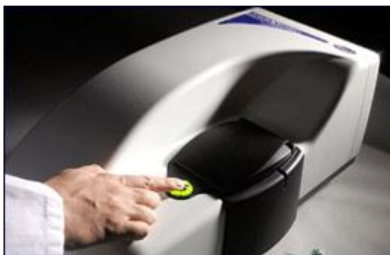
Figure 6.4: Zetasizer setup (Malvern Zetasizer Nano ZS, Worcestershire, UK).
