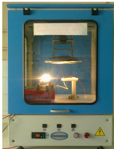
Figure 6.3: Electrospinning setup (Inovenso NE100, Turkey).
