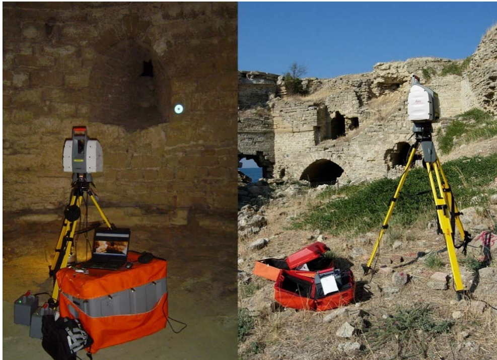
Figure 4.1 : Leica HDS 3000 terrestrial laser scanner[10].
