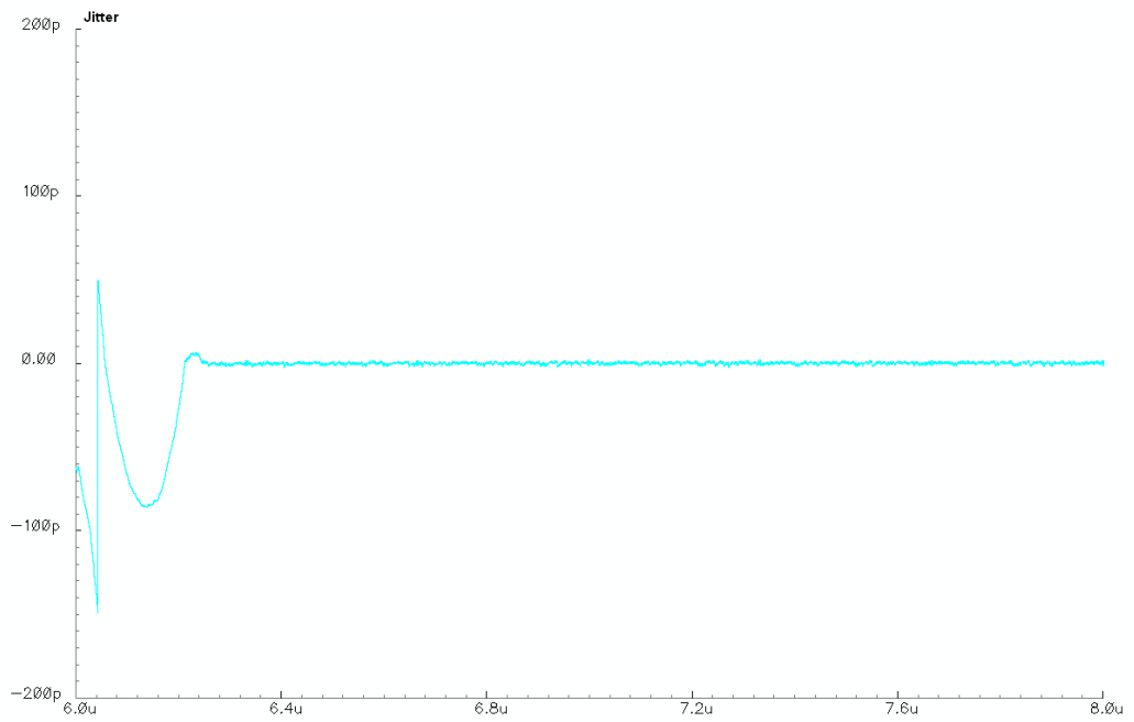
Figure 5.22: Jitter between data and sampling clock
