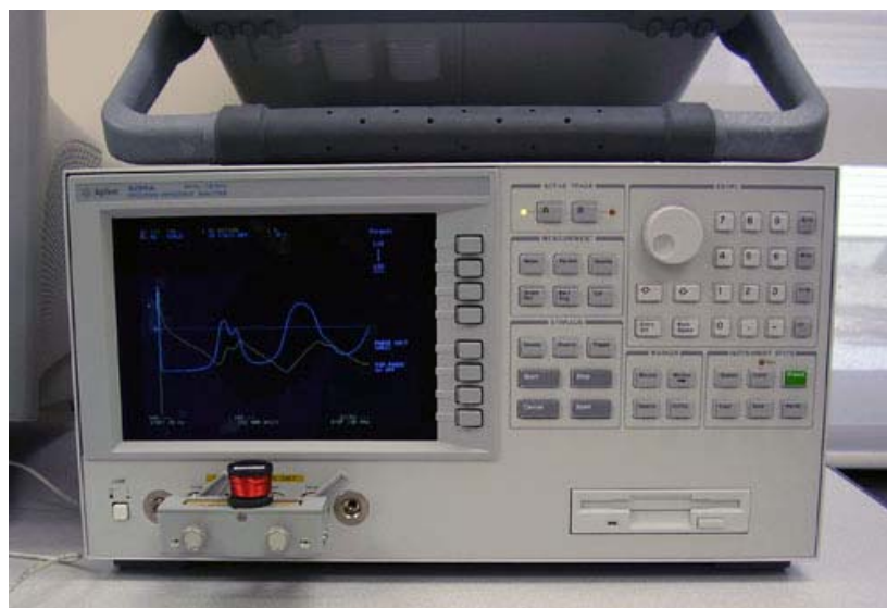
Figure 4.14: Precision Impedance analyzer (4294A) [8].
