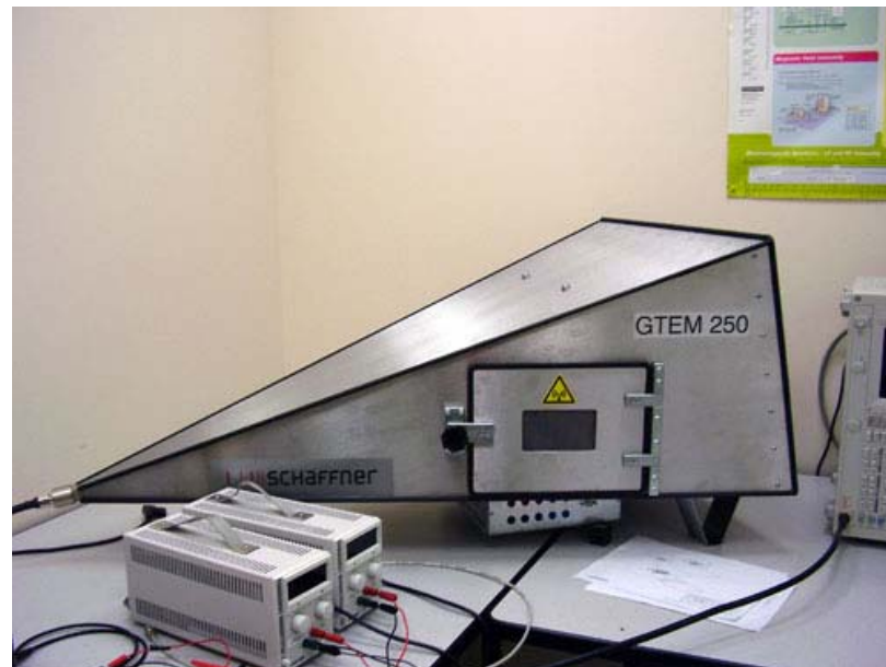
Figure 4.10: Schaffner GTEM Cell 250 for Emitted Compliance Test [8].
