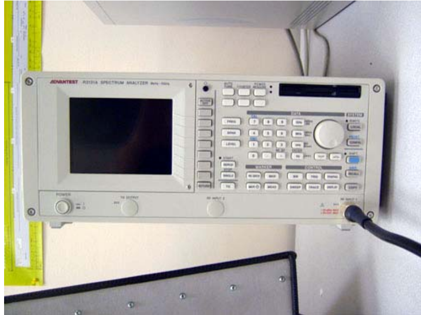
Figure 4.11: Advantest R3131A Spectrum Analyzer (9kHz-3GHz) [8].
