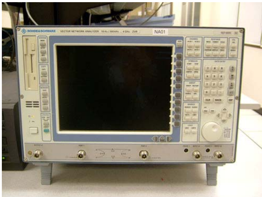
Figure 4.12: Rohde & Schwarz Vector Net. Analyzer ZVR-62 (300kHz-4GHz) [8].
