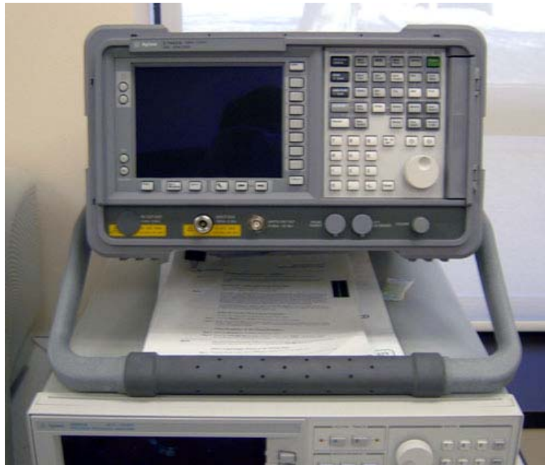
Figure 4.13: EMC Analyzer 9KHz to 3 KGz (E7402A) [8].
