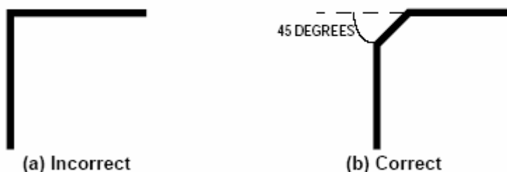
Figure 2.14: Incorrect (a) and Correct (b) PCB Track Layout [5].
