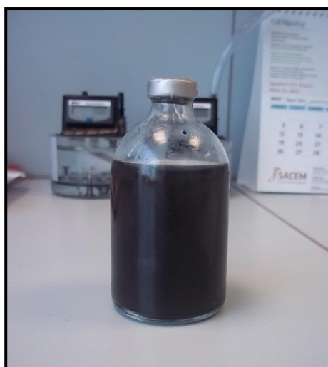
Figure 3.2 : 120 mL serum bottle with 100 mL active volume used for tests.
