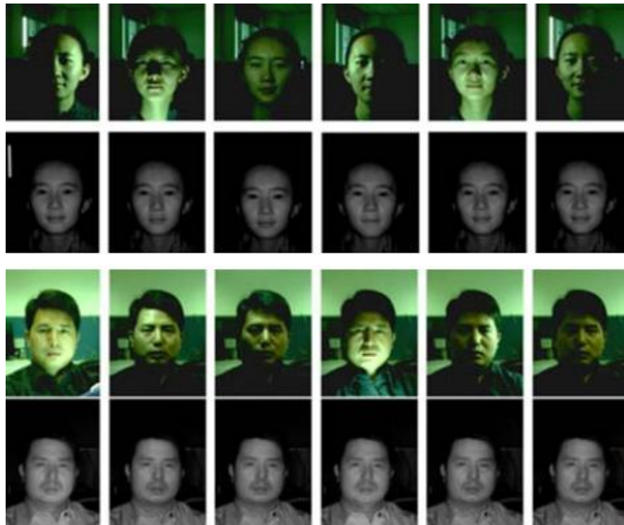
Figure 2.3 : Color images (top) captured by a color camera versus NIR images (bottom) captured by an NIR imaging system [2, 7].
