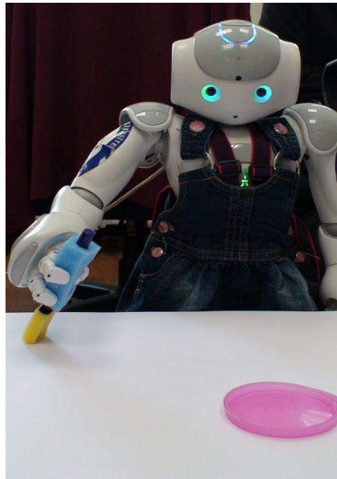
Figure 3.4: NAO blinks its eyes when the color case is in the field of vision.
