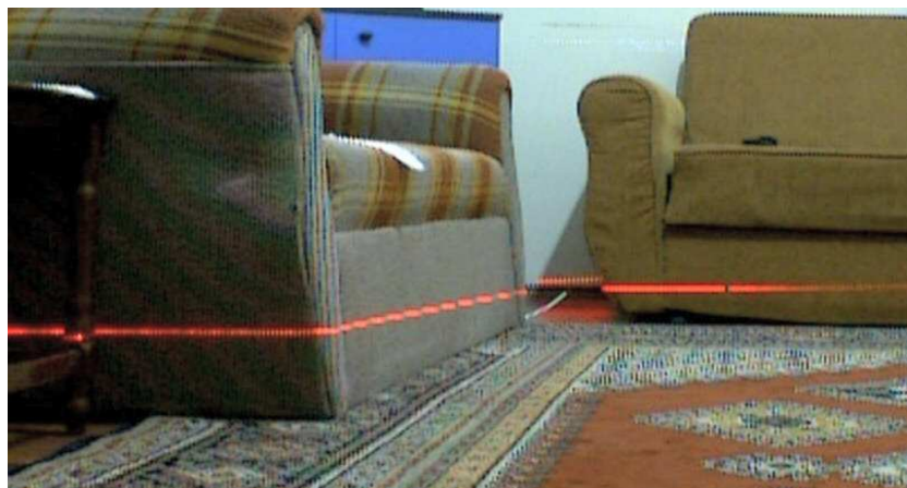
Figure 4.1 An Example of Changing of Laser’s Location on Image with Distance
