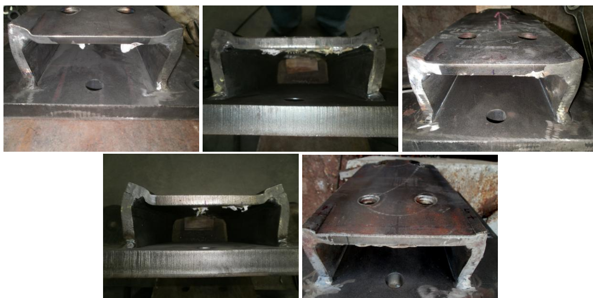
Figure 9 - Deformation on the bottom of prototypes A-11 to A-14 and A-16 in monotonic tests
