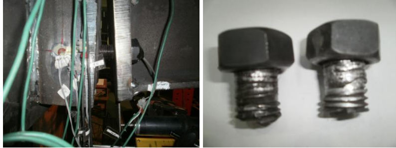
Figure 13 - Details of bolts sliding in joint A-13
