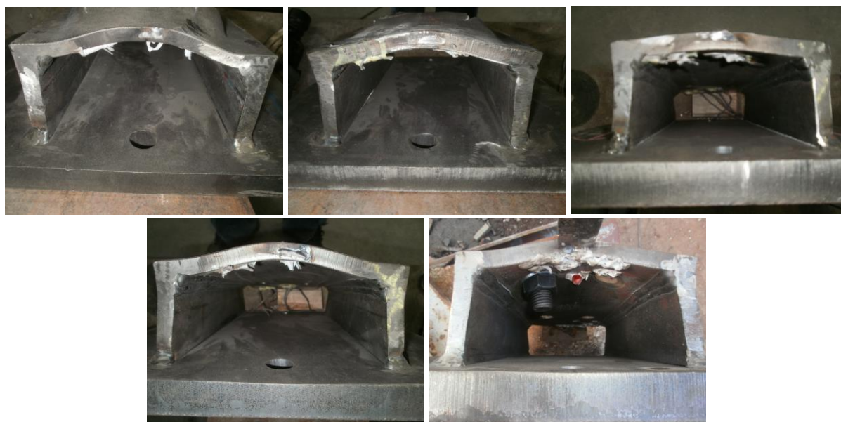
Figure 8 - Deformation on the top of prototypes A-11 to A-14 and A-16 in monotonic tests
