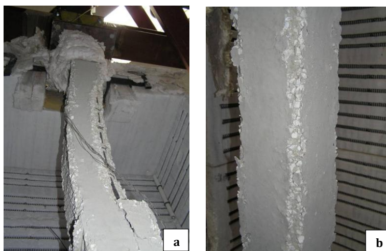
Fig.7 Columns of square cross section ( 160 \times 160\text{mm}^2 ), reinforcement ratio A_s/A_c=1.23\% .
