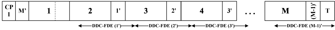
Fig. 6. Shifted length- N FFT windows for the complementary DDC-FDE procedure (T denotes the length- L required tail, preferably zero-padded).
