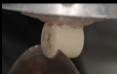
Fig. 1. Cut of the ceramic discs IPS e.max Press HT (Ivoclar Vivadent, Schaan, Liechtenstein).
