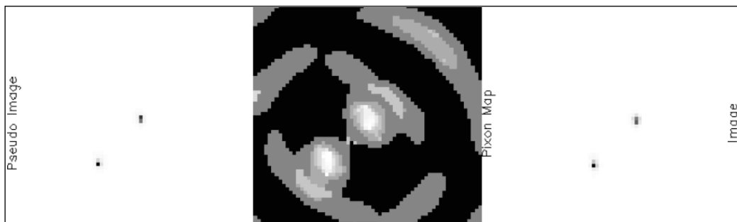
Figure 18 - Pseudo image and its correspondent Pixon map with the resulting reconstructed image. The Pixon map shows the spatial scale applied at each pixel, which represents where the information is concentrated ( 36 ).
