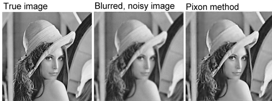
Figure 16 - Performance of the Pixon method for the “Lena” Matlab image (34).
