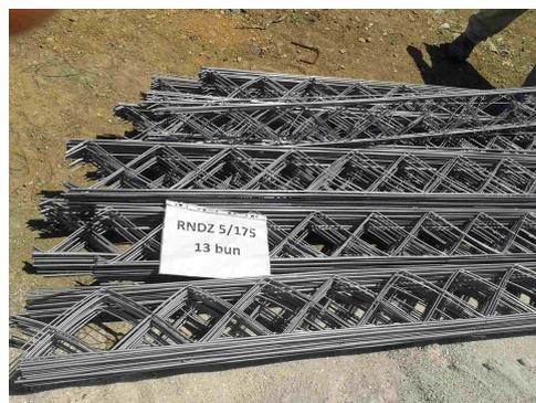
Figura 3.39: Armadura Murfor<sup>®</sup>RNDZ 5/175
