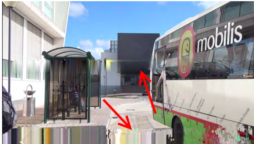
Figure F.21: Still image from ESTG Bus Stop sequence, for 1% UDP packet losses
