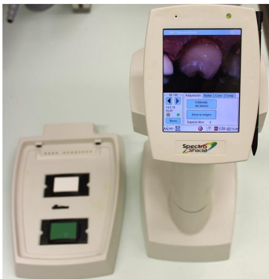
Figura 2 - Spectroshade Micro Óptic (MHT Optic Research, Niederhasli Switzerland).
